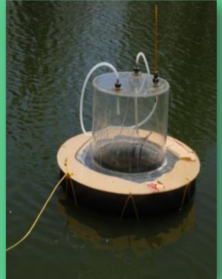
Floating chamber for collection of GHGs flux from aquaculture ponds
