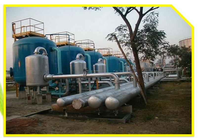
Water Filtration Plant (Capacity 720 tonnes/hour) at Jamuna Fertilizer Co. Ltd. Tarakandi, Jamalpur
